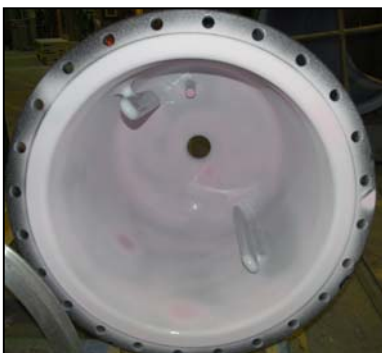
OptiMix ® 630 L: with 2 integrated baffles
